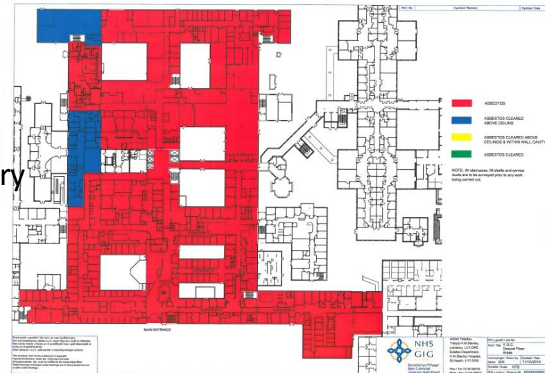
Ground Floor Asbestos Condition
